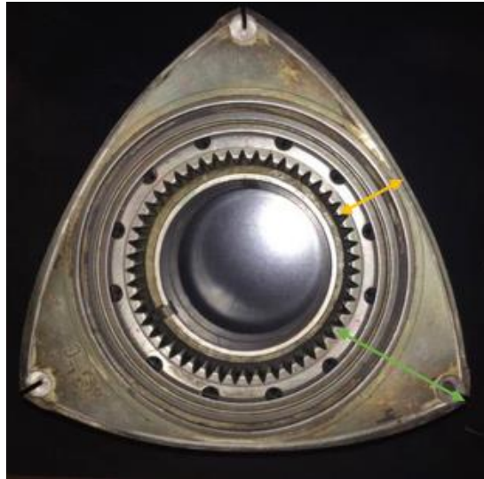
Figure 19.0.1 – Measuring value of “d” of the rotor. (Jay, 2017)
