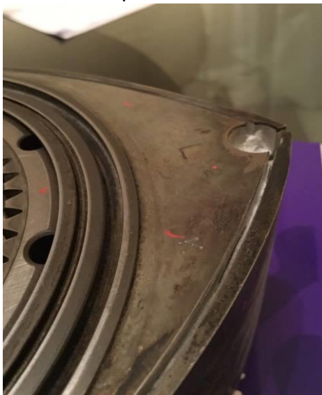
Figure 12.0.2 – Red Dots Required for CMM Scan. (Jay, 2017)
