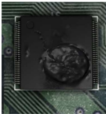
Figure 3 - ESD damage to a PCB (Peterson, 2017)
