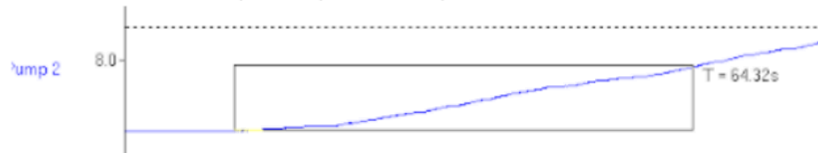
Figure 14 - Zoomed-in Graph of the Open Loop Response to the Step Change of Pump Voltage Displayed in Figure 13.
