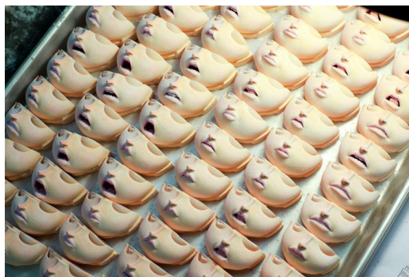
Lower face plates 3D printed for Paranorman (Grunewald, 2014)
