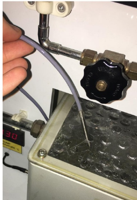
Figure 3- Sump Tank RTD
