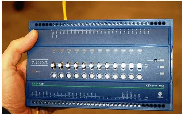
Figure 26 - DDC Controller (Instrumentation Tools, 2025)
