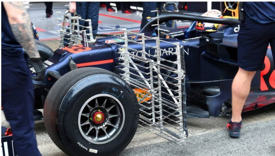
Figure 4: The Kiel Probes secured to the scaffolding forming the aero-rake. This setup is being used to measure the air flow over the wheels and linkage (Smedley, 2019).
