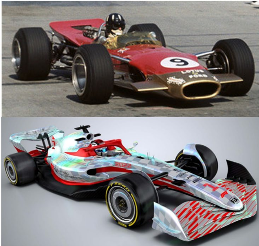
Figure 6: The first front wings (top) resembled simple inverted aerofoils (Oggioni, 2019) whilst modern front wings (bottom) utilise multiple wing elements and additional features like end plates (Stuart, 2021).
