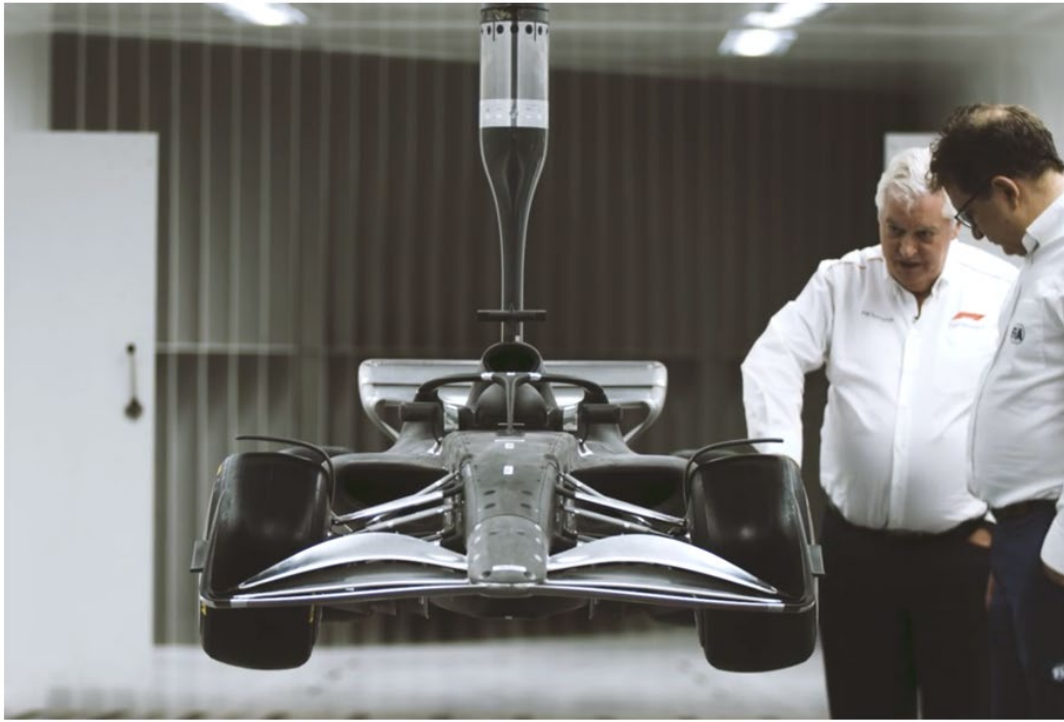
Figure 3: An intricate scale model of a F1 car to be tested in a wind tunnel. Every detail is recreated to provide the most accurate results, at a price (Stuart, 2021).
