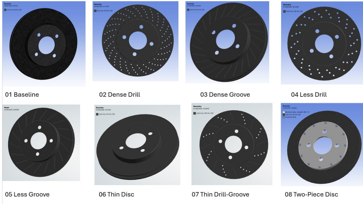
Figure 5: Eight brake-disc geometries investigated in the study.
