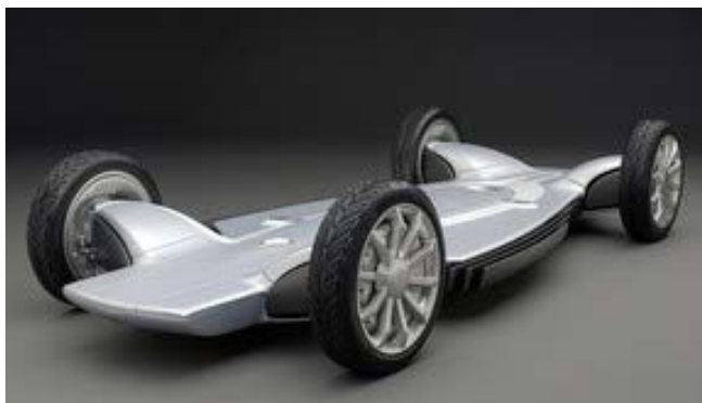
Figure 9. Electric Vehicle Skateboard (McIntosh,2020,p.1)
