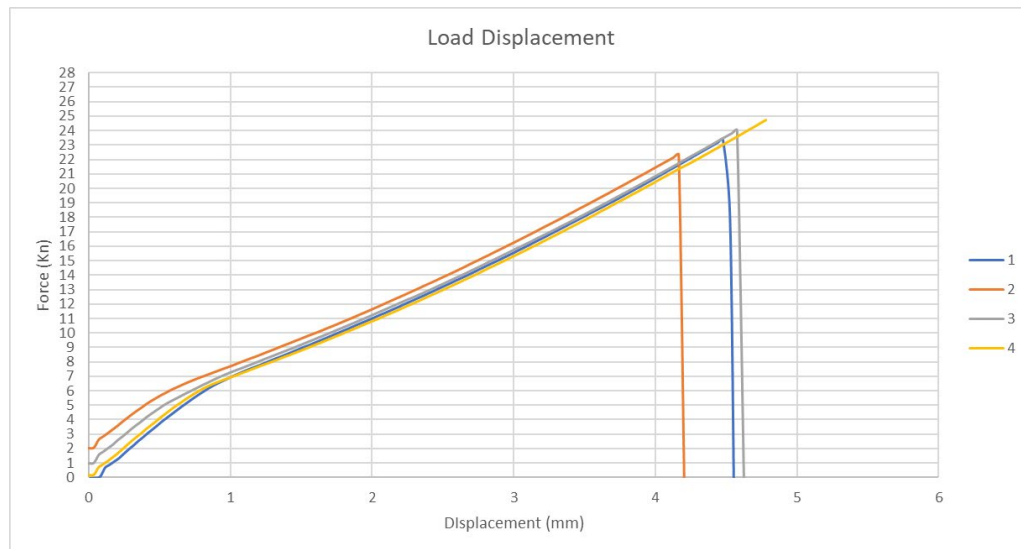
Figure 39 – Easy composites 0° UD load displacement chart
