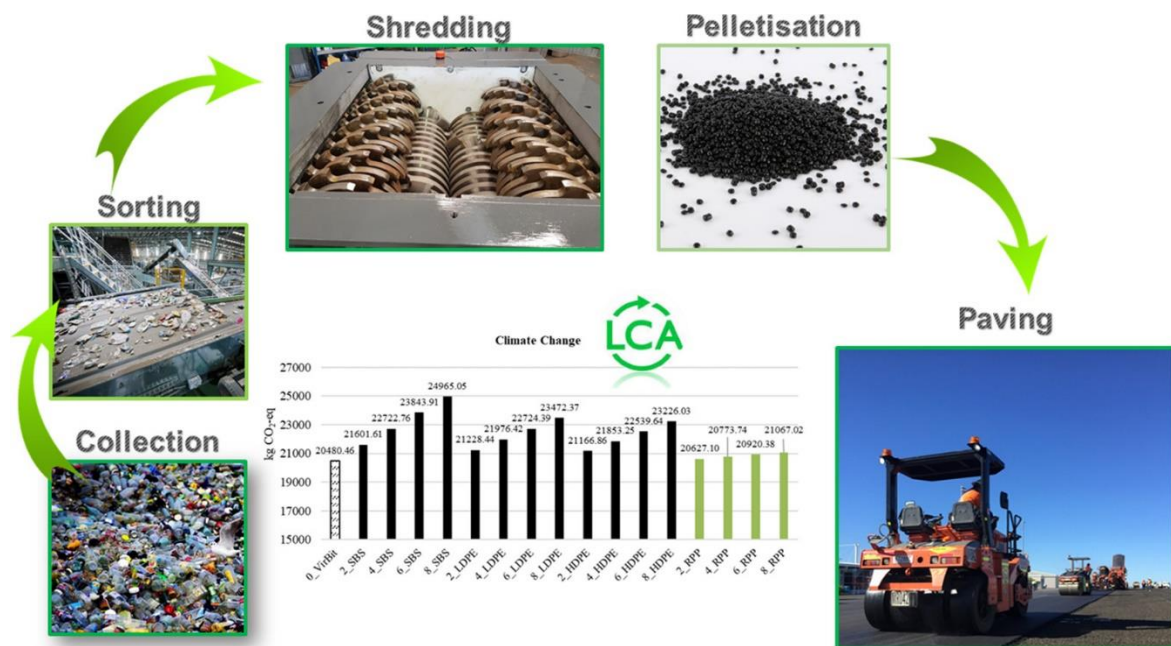
Image 1 Recycling waste plastic for use in infrastructure like roads. (Science Direct, 2021)
