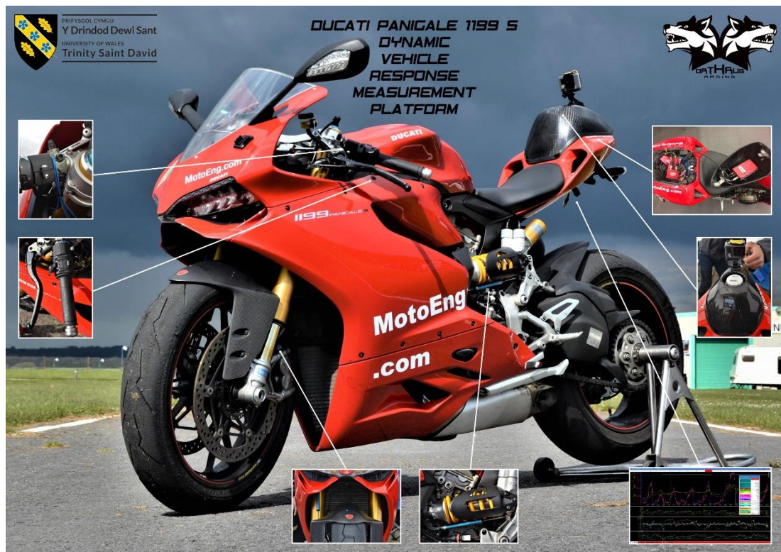
Figure 3 The DVRMP along with its aftermarket sensors and custom-built features
