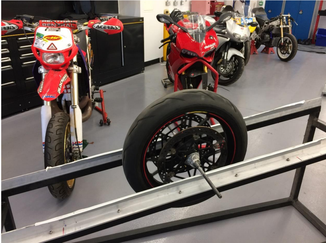
Figure 11 Picture of experimental procedure to determine the front wheel spin inertia
