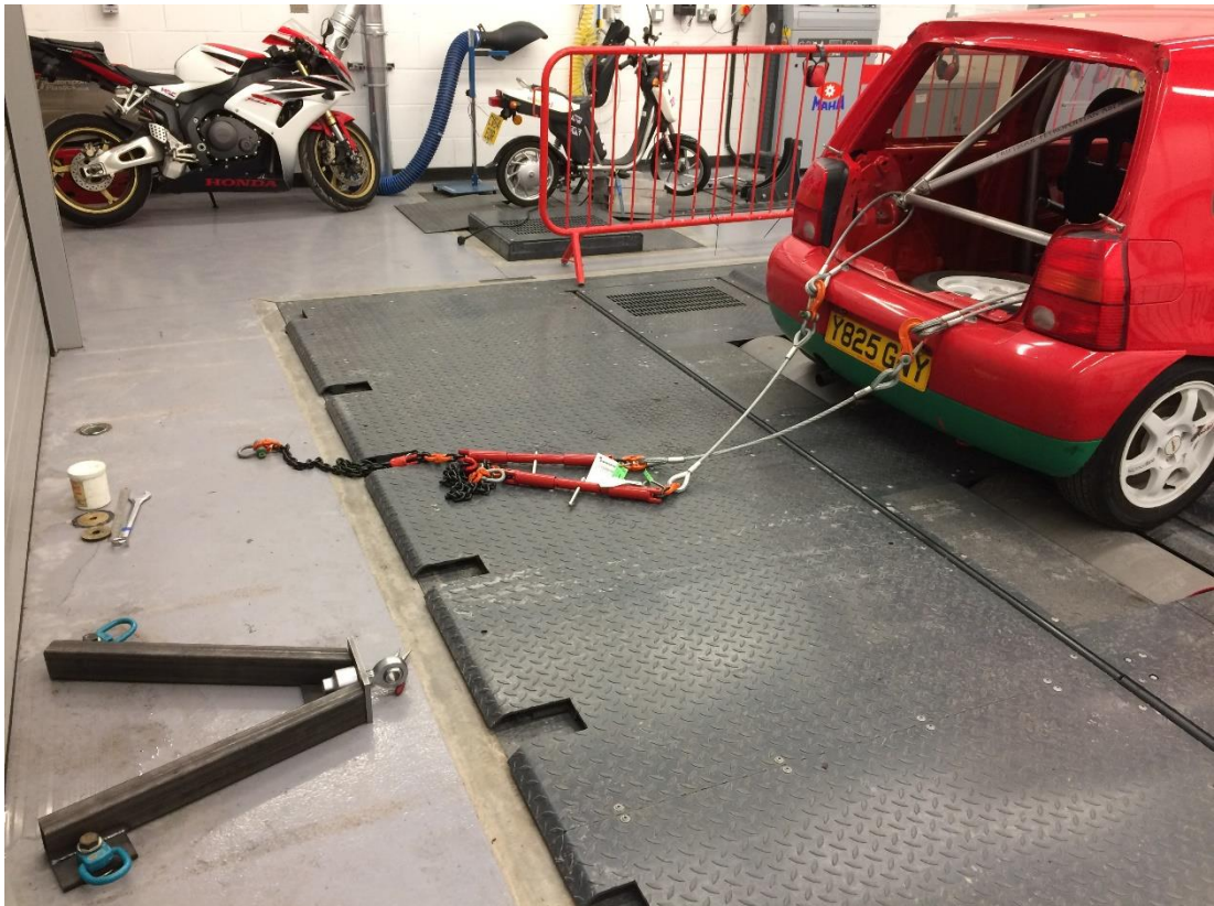
Figure 14 Picture of the bottom part of a rig for possible step-tests on a car dynamometer
