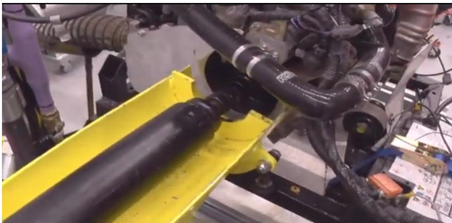
Figure 1 (Honda VTEC 1.6 Engine attached to Dynamometer via Drive Shaft)
