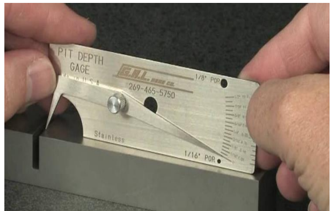
Figure 12: An example of Pit gauging, [53]
