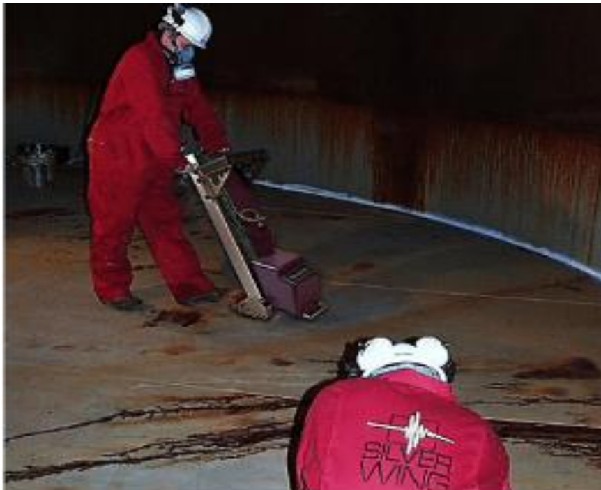
Figure 4: Out-of-service tank floor inspection with floormap in hazardous tank environment. Image provided by Silverwing (UK) LDT. [8].
