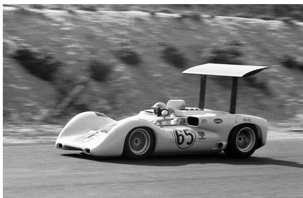
The Chaparral 2E, which raced in the 1966 Can-Am series, was unlike any other competitor, due to the large rear wing mounted 4ft above the rear decklid. This rear wing generated 110kg of downforce at 100mph. (Barlow,2016)
