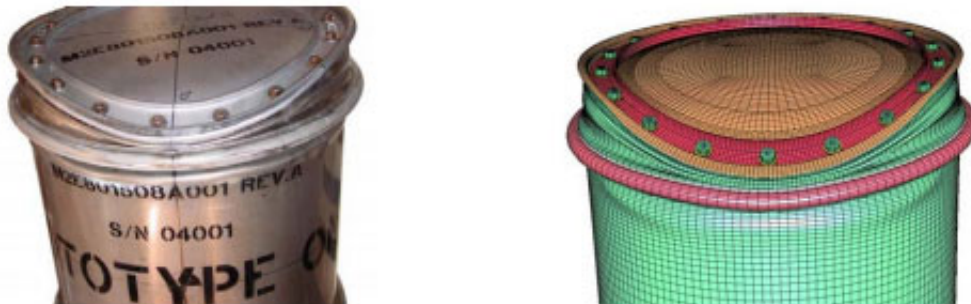
Figure 2-5 Comparison of deformation of a shipping package of FEA vs real life
