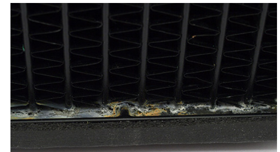
Corrosion in Radiator (MartinsLiquidLab, 2012)
