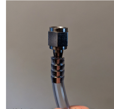
1/8 in Female BPSS to 7mm barb. This end was used in vacuum generator.
