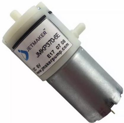
Cheap Diaphragm Pump ~£1 to £5 Max pressure ≤560hPa Lifespan >500 hours (Alibaba, 2022)
