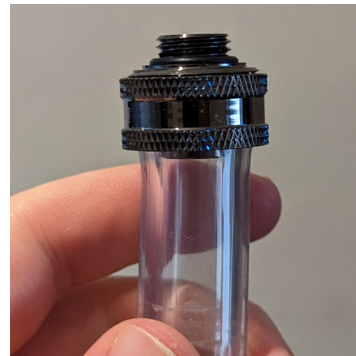
Once fitted, I was unable to remove it, even when unscrewing the compression fitting.
