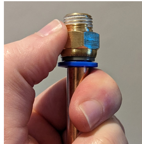
Applying force to try and push off brass fitting. It did not move at all.
