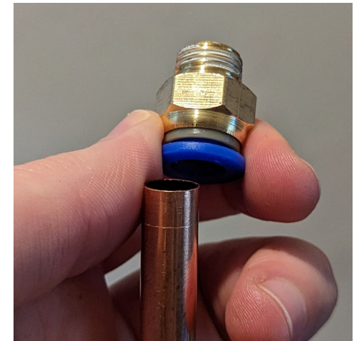
When force applied to blue plastic it quickly comes off, leaving a score mark on pipe. (will this be okay after multiple removals?)
