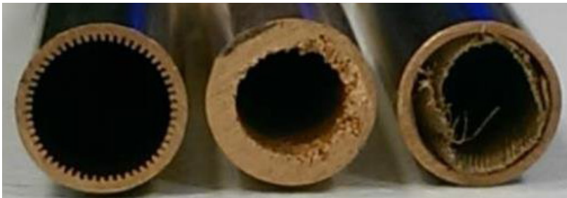
Heatpipe cross-section of axial grooved, sintered and mesh. (Alshehhi, 2019)
