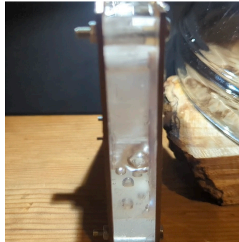
In the first 2 minutes the air trapped in the water was pulled out
