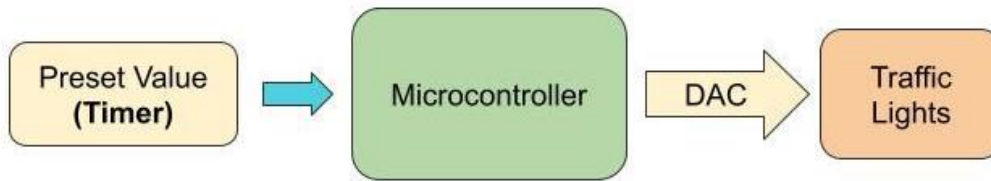
Figure 5: Traffic Light Open Loop Model. Source: Adapted from [5]
