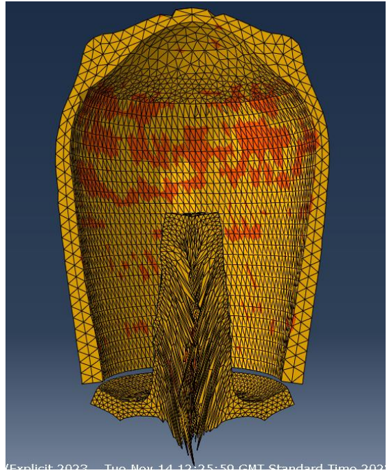
Figure 31 - Formation of jet - Can see Liner is not constrained to Casing and follows the jet
