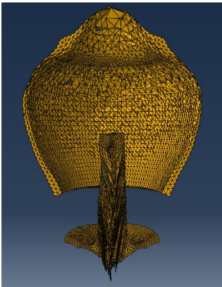
Figure 32 - Further formation of jet. Good blast
