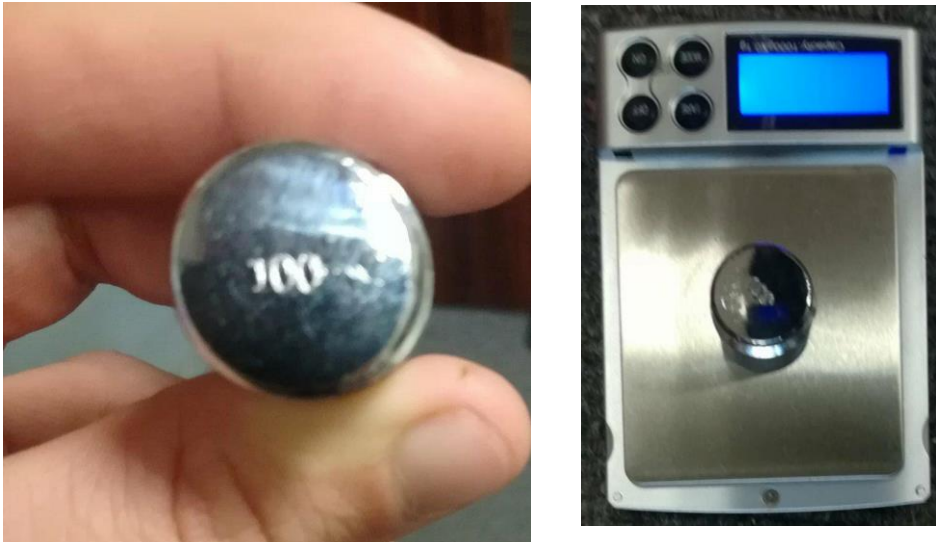
The 100 gram calibration piece measured in at 100.01 grams
