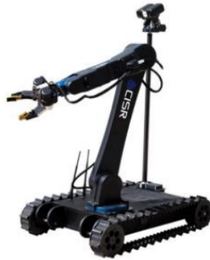
Figure 2-1 Haptically-Enabled Counter IED robotic system [5]
