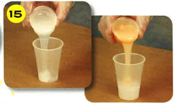
The Dragon Skin® FX-Pro® Part A and B are combined in a clean mixing cup.
