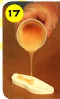
Dragon Skin® FX-Pro® is poured into the mould, and excess silicone is scraped off using a wooden mixing stick.
