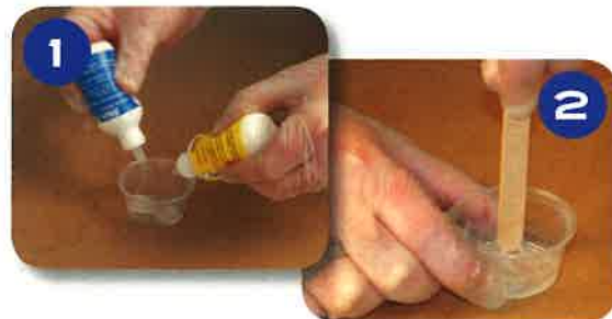
Skin Tite® silicone adhesive is measured 1A:1B by volume and thoroughly mixed.
