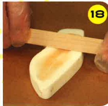
Dragon Skin® FX-Pro® is poured into the mould, and excess silicone is scraped off using a wooden mixing stick.
