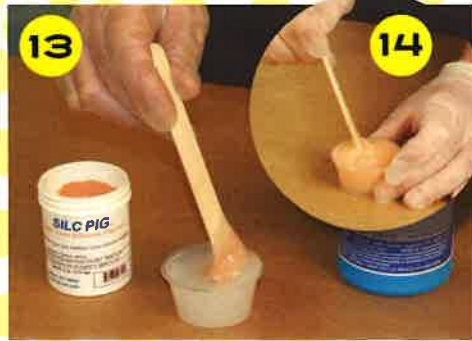
The FX-Pro® part B is pigmented using Silc-Pig® fleshtone and pre-mixed.
