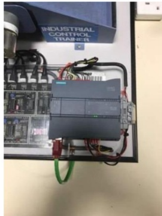
Figure 6 - PLC utilised on the trainer
