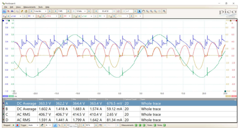
Appendix Figure 28 - Constant Torque / Variable Speed in Quadrant 1 – 2000rpm
