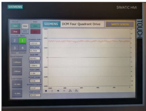
Appendix Figure 30 - Practical - Varying Torque / Constant Speed 2000rpm/6.66Nm HMI
