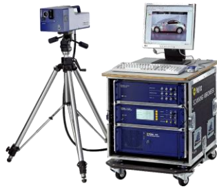
Figure 2: PSV 400 Data Management system & Scanning head (NetScope Solutions)
