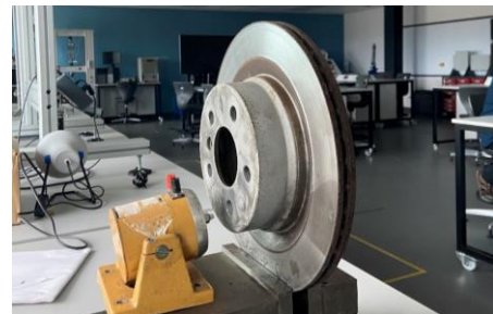
Figure 1: Brake disc and Solenoid used for Measurement. (Iatrakis, 2024)
