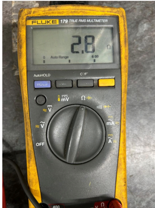
Figure 25 - Test 1 - Continuity of Earthing Conductors
