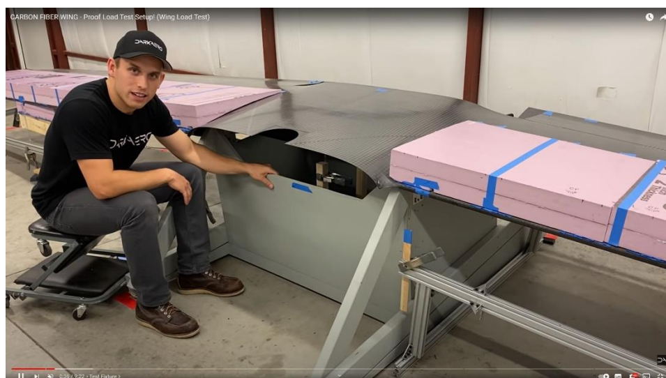
Fig 7.0: Highlighting basic carbon fibre deflection test, of air plane wing to scale (Aero, 2021)
