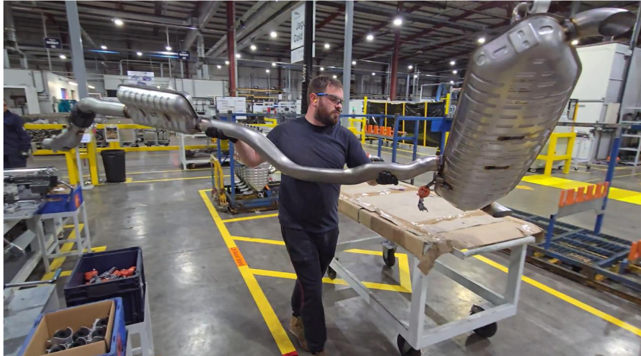
Operator manually handling the P6 MHEV exhaust assembly between leak testing and packaging operations.
