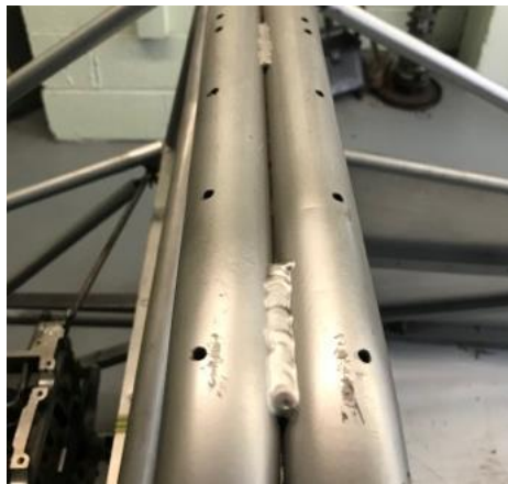
Figure 14 Roll hoop welds
