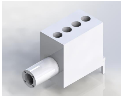
Figure 16 Rendering of engine block and gearbox for FE model
