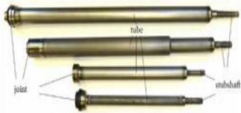
Figure 8 – Subshafts used in automotive industry (Kustroń, et al., 2017)
