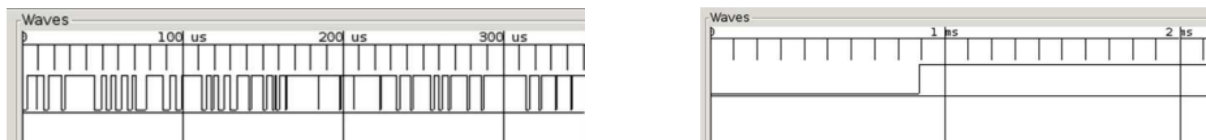
Figure 3.6 – Bouncing Waveform Versus Ideal Debounced Switch
