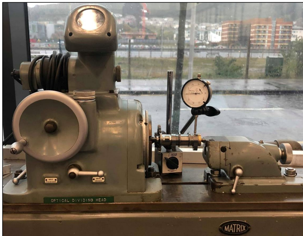
Figure 51 Measuring KTM Moto3 Cam-Profile with Optical Dividing head
