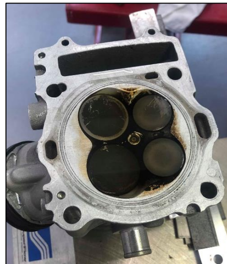
Figure 37 KTM Inclined Valve Alignment
