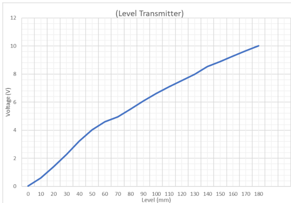
Figure 6; Calibration Curve Level Transmitter
