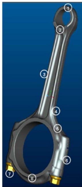
Figure 5 – Critical connecting rod sections
