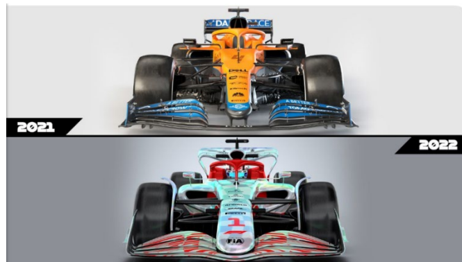
Figure 7 - 2021 vs 2022 Front Wing
