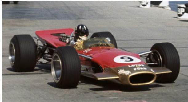
Figure 5 - Lotus Front Wing Introduction 1968
