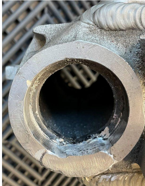
Figure 14 Photograph of weld on steering column (F. Flye, 2025)
