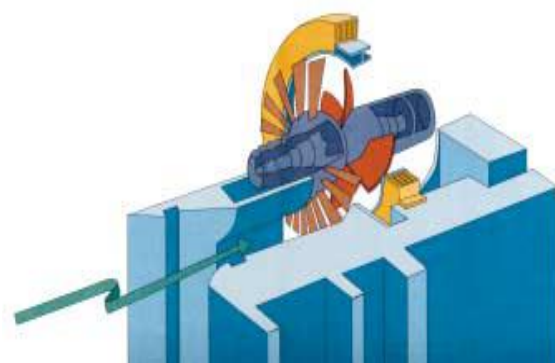
Figure 13-Straflo Turbine used in Annapolis TPP (Electrical Line Magazine, 2002)
