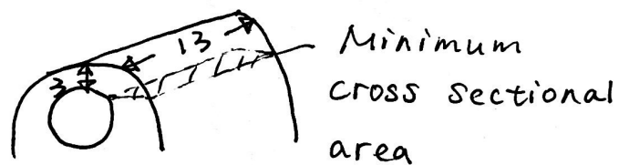
Figure 4.2 Minimum cross sectional area
