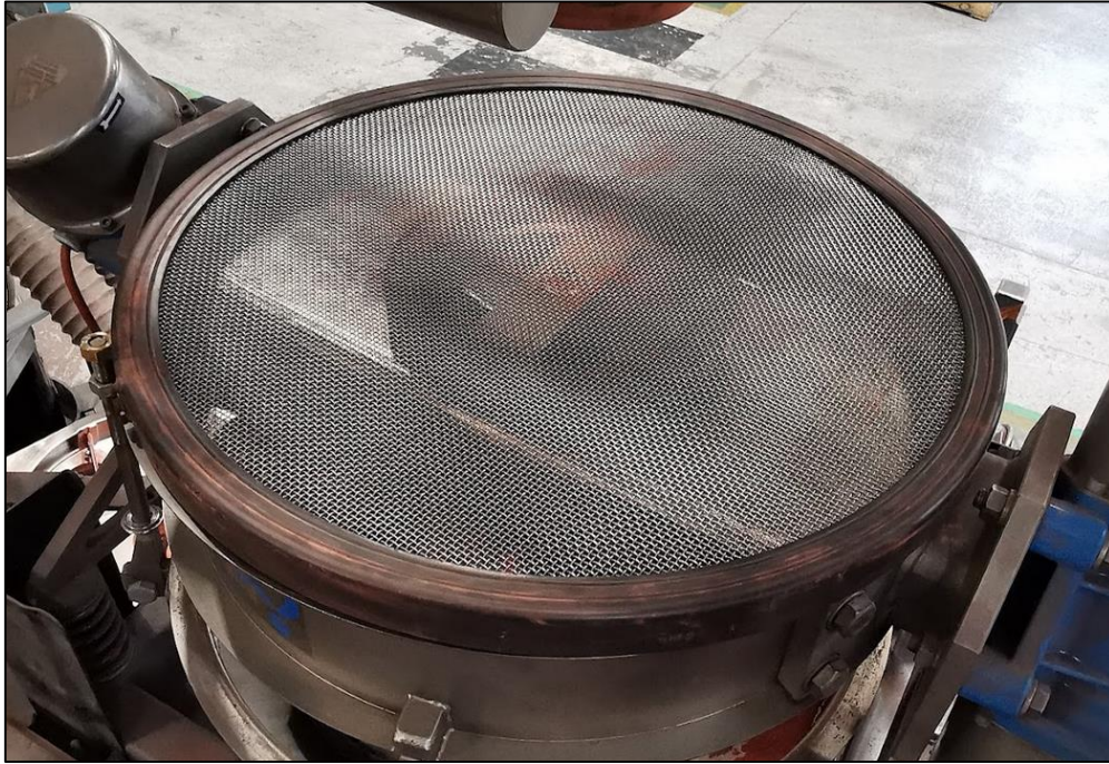
Figure 10 - Multi-frequency Sieving Machine Without Working Mesh
