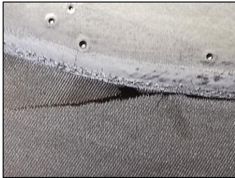
Figure 7 - Mesh Fracture from Impact
