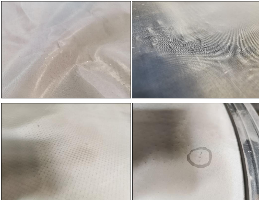
Figure 9 – Examples of Unique Wear on Multi-frequency Sieves
