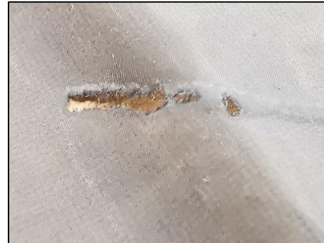
Figure 8 – Mesh Fracture from Work Hardening
