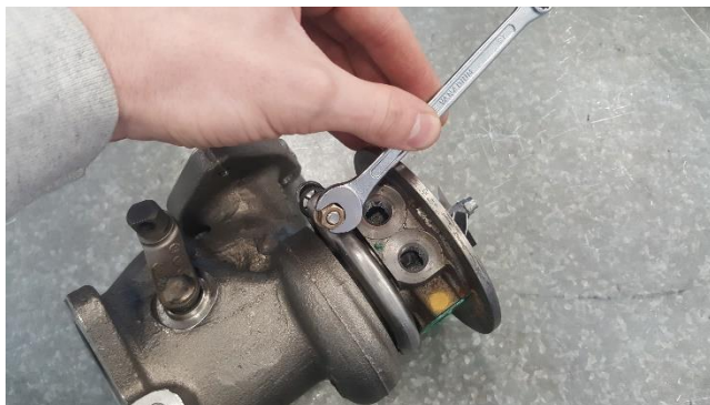
Appendix 20 – Turbine housing removal (Kot, 2019)
