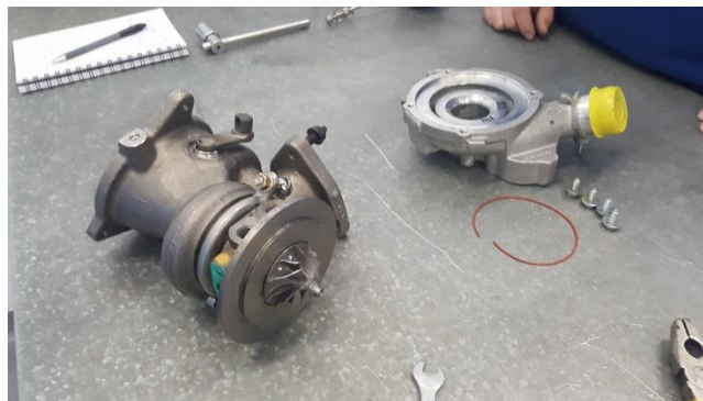
Appendix 20 – Turbine housing removal (Kot, 2019)
