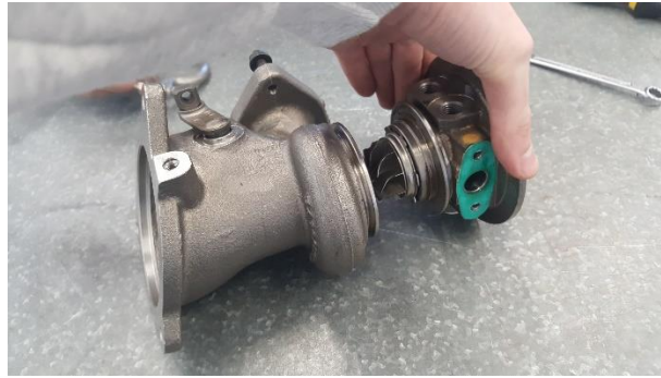
Appendix 22 – Turbine housing removal (Kot, 2019)
