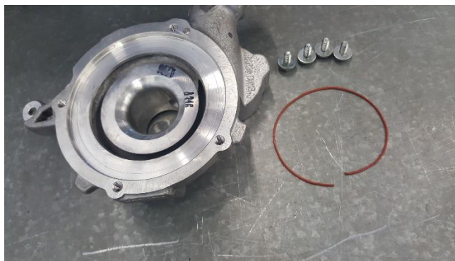
Appendix 19 – Compressor housing removal (Kot, 2019)
