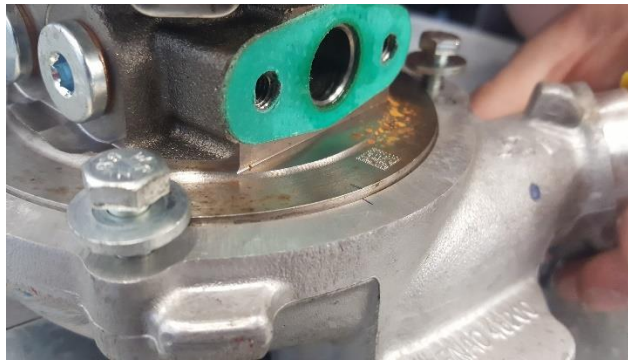
Appendix 18 – Compressor housing removal (Kot, 2019)
