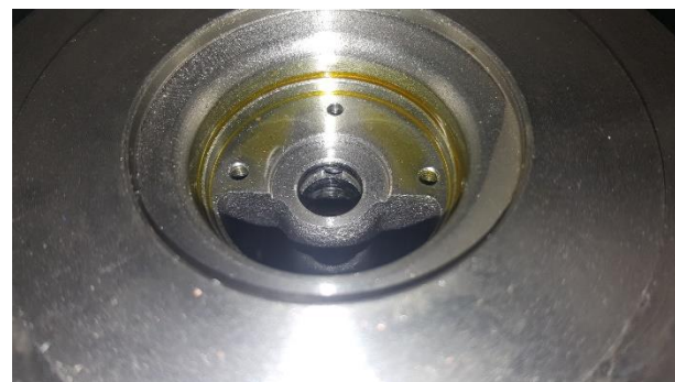
Appendix 32 – Oil galleries within the housing (Kot, 2019)
