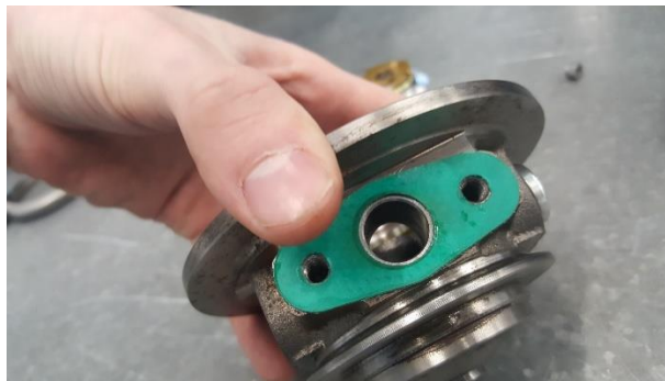
Appendix 35 – High pressure oil pipe fitting on housing (Kot, 2019)
