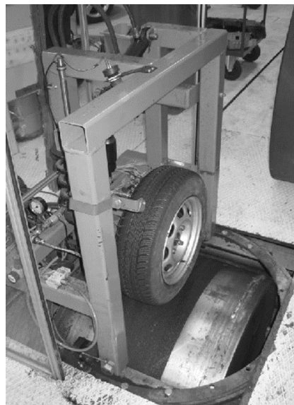
Figure 9: Tyre Testing Rig used for FE development (Korunović*, Trajanović, Stojković, Mišić, & Milovanović, 2011)
