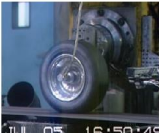
Figure 12: Calspan Testing Machine on Avon FSAE Tyres (Kasprzak & Gentz, 2006)
