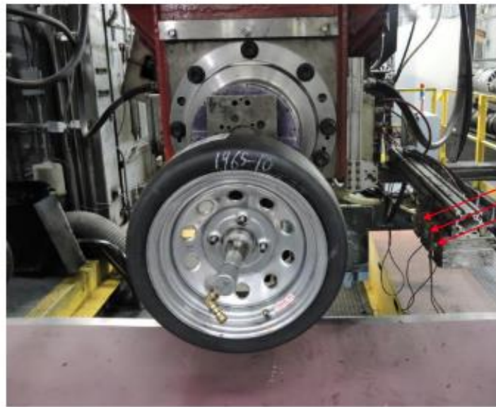
Figure 14: Rig used on Round 9 of FSAE TCC testing (FSAE Tire Test Consortium, 2022)
