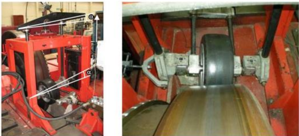
Figure 8: Tyre Testing Rig (Garcia-Pozuelo, Yunta, Olatunbosun, Yang, & Diaz, 2017)
