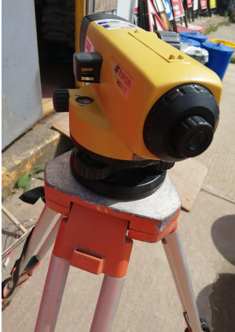
Figure 6 Top Con AT-B4 Automatic Level
