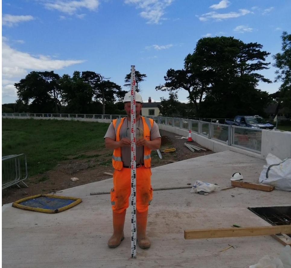
Figure 5 Chain person holding levelling staff
