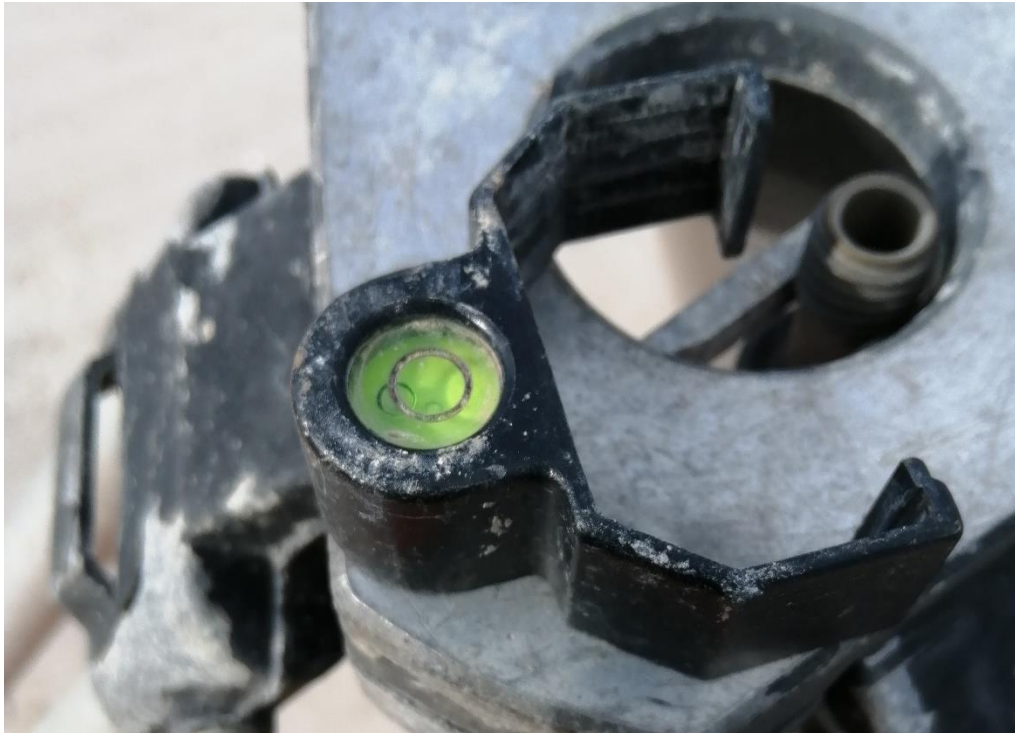
Figure 4 Plumb bubble that can be clipped to a levelling staff
