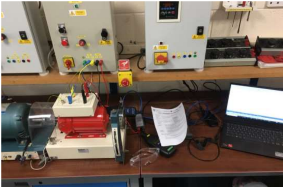
Figure 26 - Practical investigation into a Single quadrant DC Drive - Practical Setup
